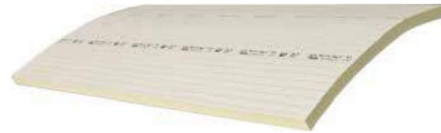
Insulation core: PUR/PIR rigid foam in accordance to DIN EN 13165, class E, with mineral fleece on both sides, insulation element slit above and below Edge connection: round about edgeless. Please note: Vapour barrier to be fitted on site. When constructing the roof substructure and the entire roof system the specialist rules must be observed. Identification according to EN: PUR-EN 13165-T2-DS(TH)9-CS(10\Y)100 Overall dimension: 2440 x 1200 mm (= calculation measurement)
