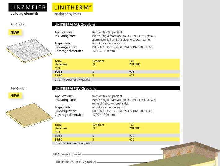
LINITHERM PAL or PGV flat roof insulation -
